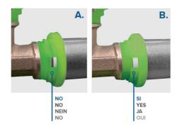
The picture "A" shows a non-correct introduction of the pipe into the fitting. The picture "B" shows a correct introduction of the pipe that is in correspondence of the head of the plastic ring.
